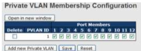
Figure 65: Private VLAN Membership Configuration
