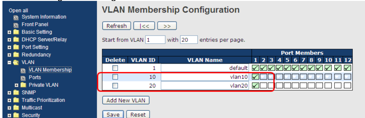
Figure 59: VLAN ID 10 & 20 VLAN Membership Configuration
