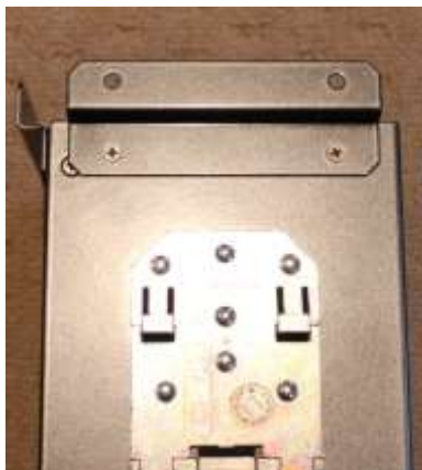
Figure 6 - Brackets Mounted on back of Switch
