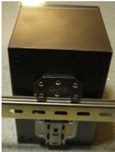
Figure 4 - Switch Mounted on DIN-Rail
