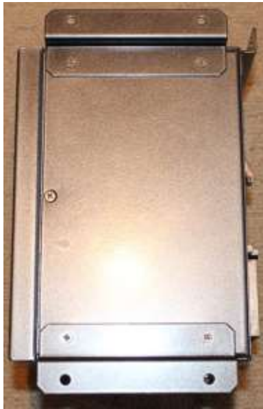
Figure 5 - Brackets Mounted on Side of Switch
