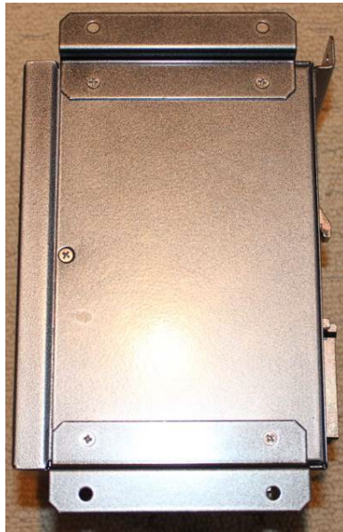
Figure 5 - Brackets Mounted on Side of Switch
