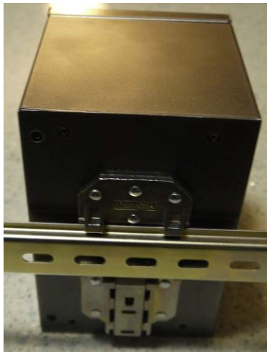
Figure 4 - Switch Mounted on DIN-Rail
