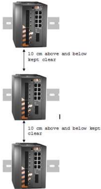
Figure 3 – Distance for Natural Air Flow
