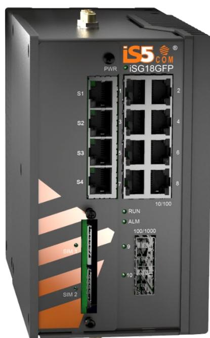
The iSG18GFP is a natural fit for installation at MV/LV transformer sites acting as secure access points for the Distributed Automation control of remote sites. This product is as a secure gateway for Ethernet, IP, and Serial services as an optimized platform for servicing these needs over the network core. The iSG18GFP provides maximum protection against cyber threats.
