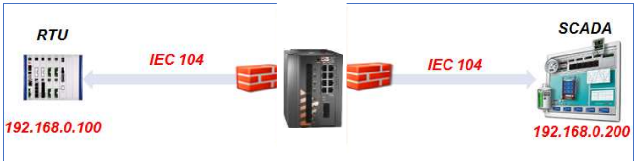
Figure 27 – Firewall Flow Illustration
