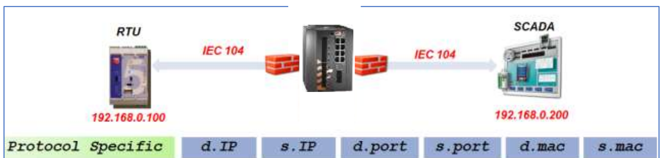
Figure 28 – Firewall Flow Illustration – Protocol Specific
