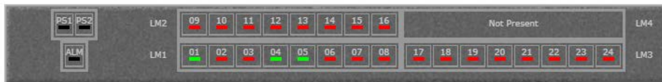
Figure 5: Port layout on the RAPTOR
