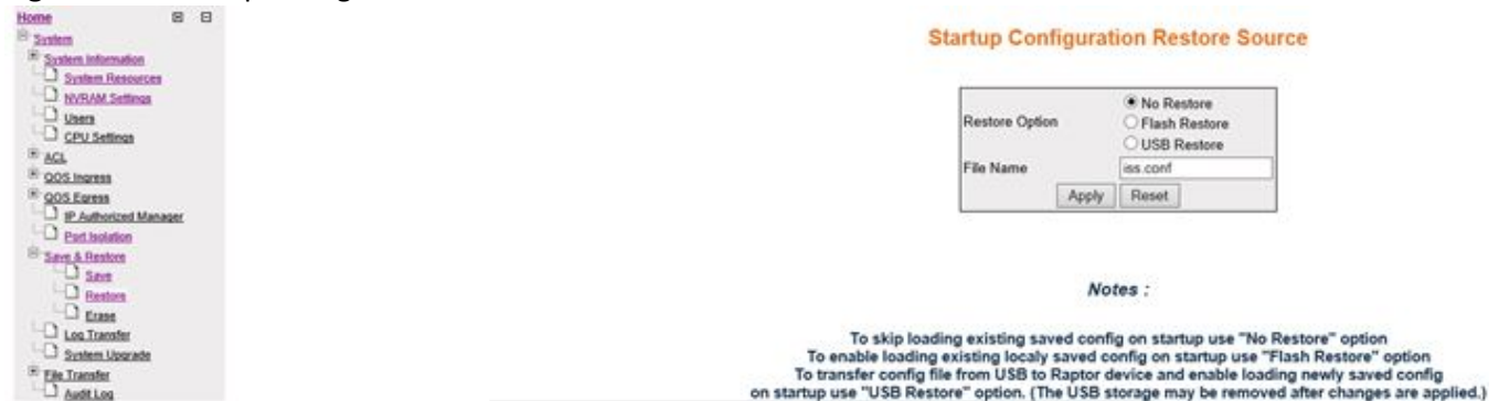
Figure 1: Startup Configuration Restore Source
